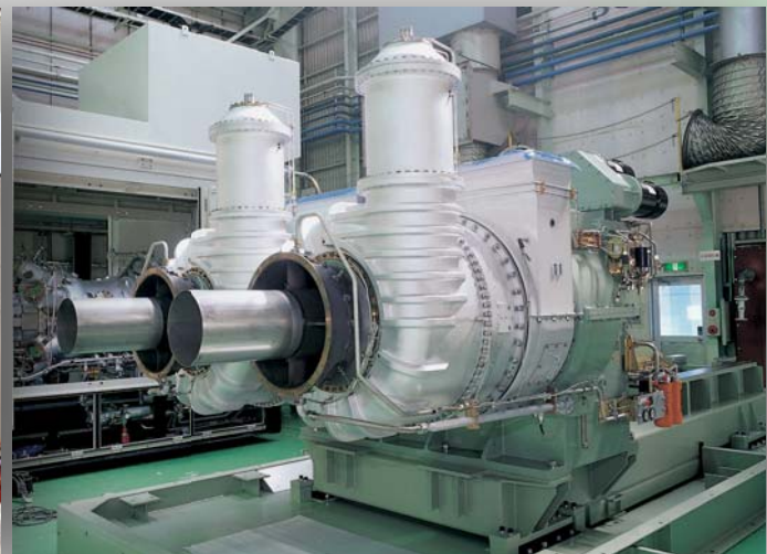
GPS4500 Generator Set for Data Center Use
