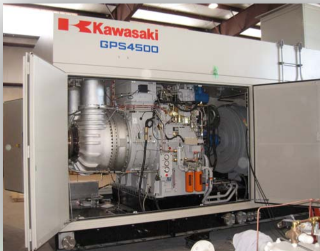
GPS4500 Generator Set for Data Center Use
