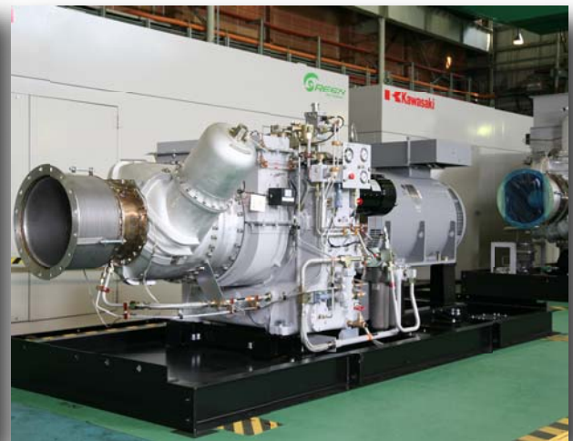
GPS750 Engine Generator Assembly 600kW on Factory Floor
