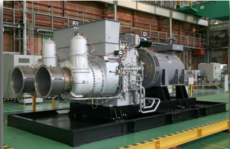
Kawasaki High Torque, Quick Start GPS Gas Turbine Generator Assembly
